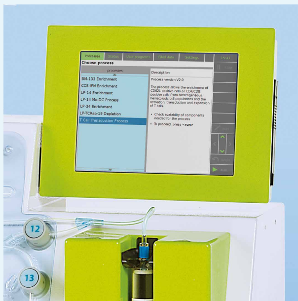
Figure 6: Touch screen for operational control of the device. The integrated FPS allows flexible programming of processing modules.
